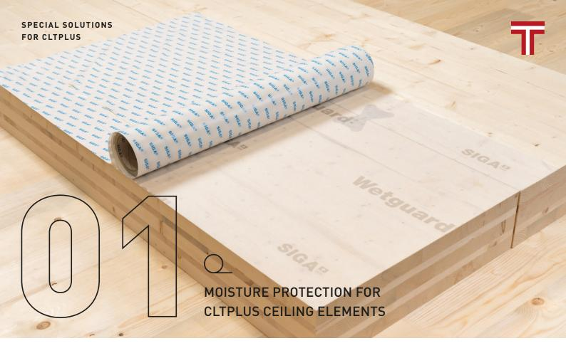
Visible ceiling elements in particular require special attention during production, transport and assembly. A specially designed, self-adhesive membrane ensures effective moisture protection on the construction site. The membrane is fully bonded to the CLTPLUS ceiling elements in the factory.
