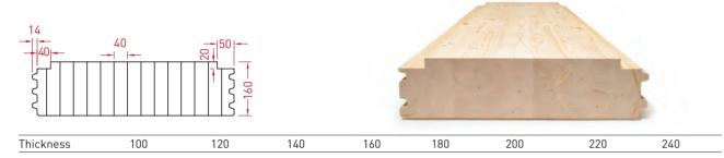
Covered dimensions: 580 mm | Invoiced dimensions: 600 mm | Groove: 14 mm | Rabbet above: 20 x 40 mm and 20 x 50 mm
