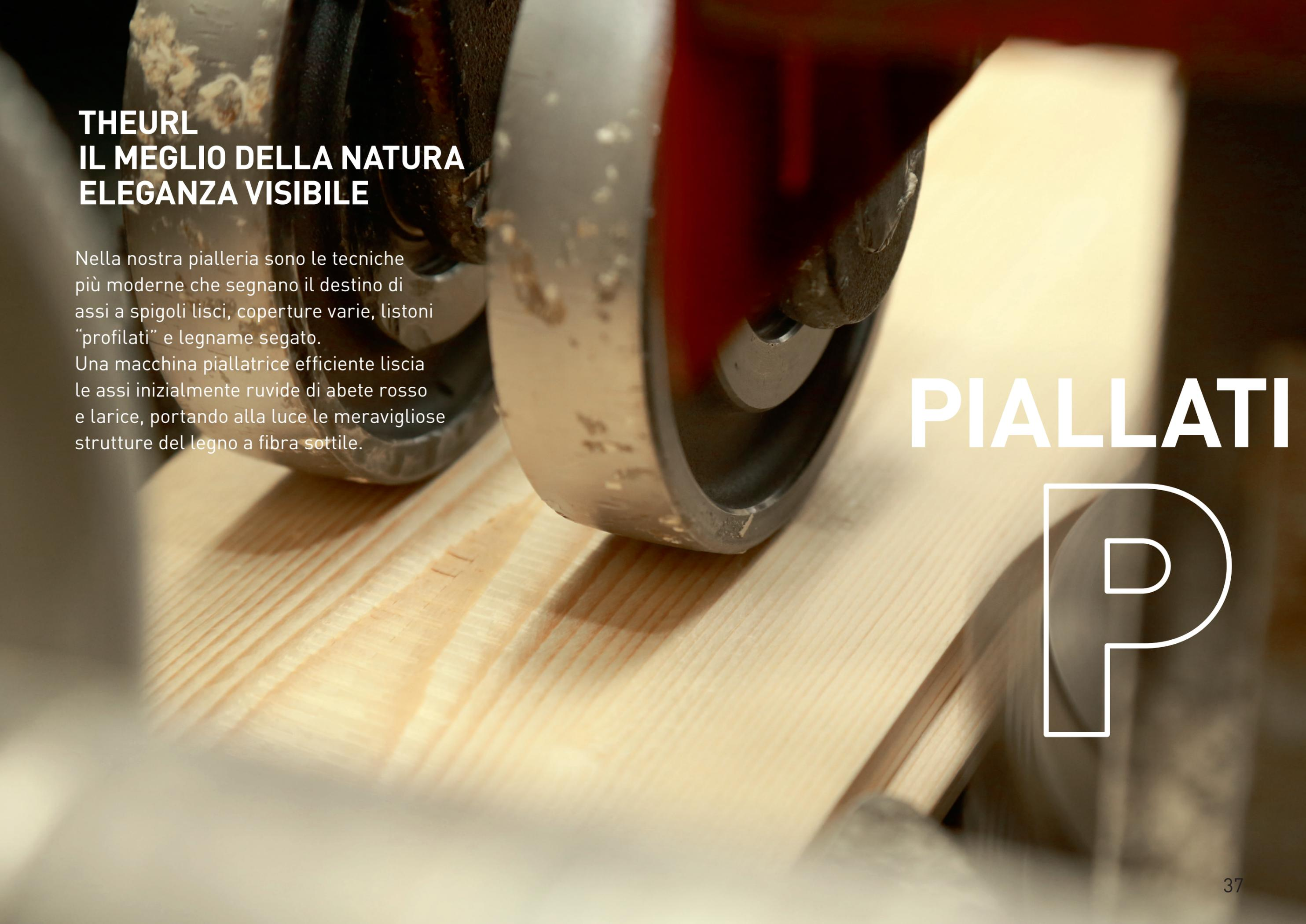
A close-up photograph of a wood planer machine in operation. The machine's rollers and blades are shown smoothing a piece of light-colored wood. The background is blurred, focusing attention on the machine and the wood. The text is overlaid on the left side of the image.
